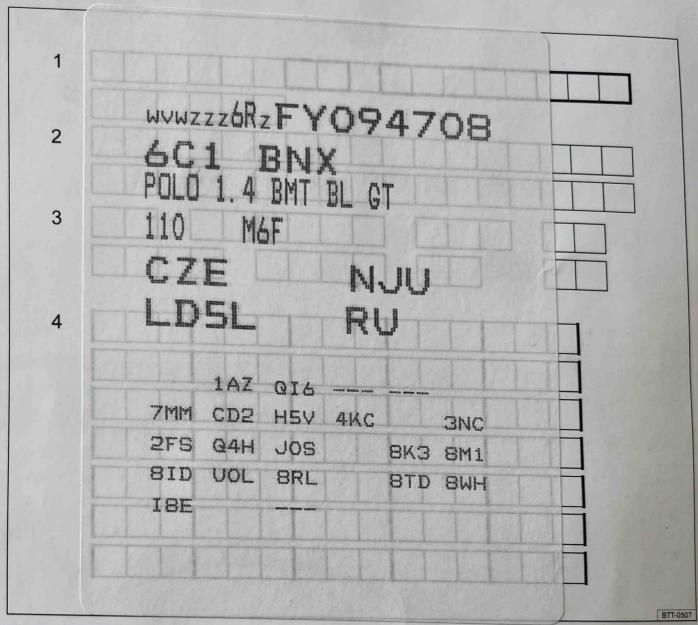
**Fig. 1** 1: Vehicle identification number; 2: Vehicle type, engine power, gearbox type; 3: Engine code, gearbox code, paint number, interior equipment; 4: Optional extras, PR numbers
